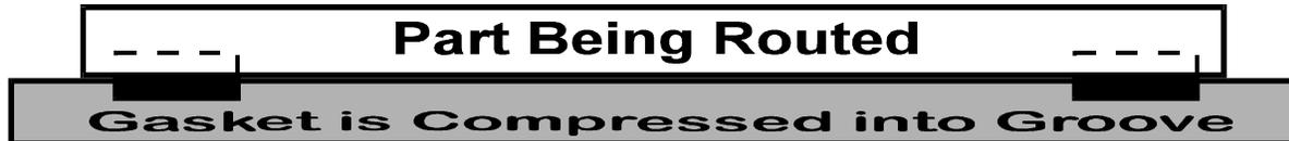
**Gasket is Allowed to Compress into Groove and Allows Part to Seat on Spoilboard Like a Platen, thus Deadening Vibration of the Part**
